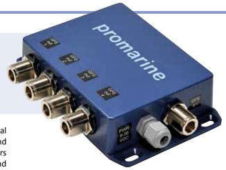
The operation is simple and reliable. proGPS™ splitters distribute GPS/GNSS antenna signal from one ideally located GPS/GNSS antenna to up to four independent navigation receivers maintaining complete galvanical and radio frequency isolation between receivers preventing one faulty receiver to interfere with others. Thus proGPS™ improves performance of a single GPS/GNSS receiver and minimizes the occupied space on the ship's topside.
