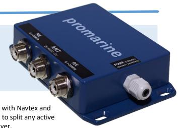
proFIL 1322 splits an active Navtex antenna (0.1MHz-30MHz) with Navtex and WeatherFax receivers or MF/HF DSC receivers. It can be used to split any active Navtex antenna that tolerates +10VDC voltage from the receiver.
